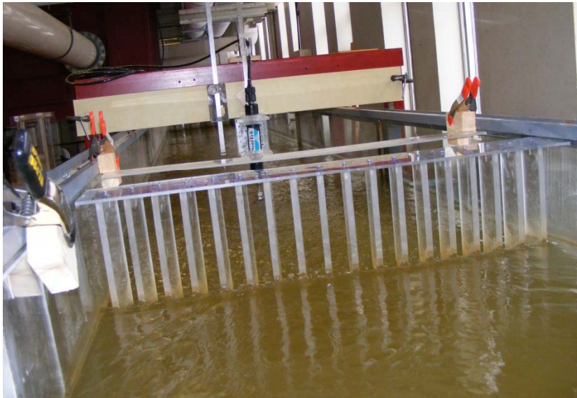
Trash rack in open channel
